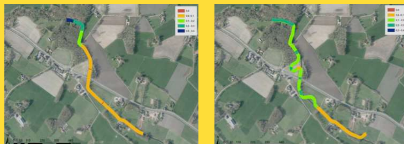
Figure 8. The flow velocities in Boven Slinge brook before (left) and after removal (right) (source: Rijn en IJssel water authority, 2016).
